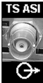
Fig. 10.9. TS-ASI connector (75 Ohms, BNC)
