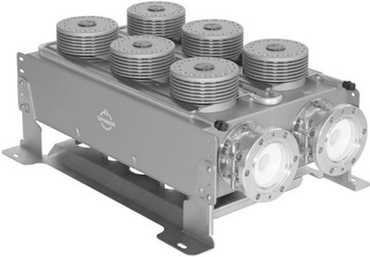
**Fig. 46.49.** Liquid-cooled, 6-circuit mask filter, non-critical mask, 7.5 kW, (3.75 kW without liquid cooling), 6, 7, or 8 MHz bandwidth, manufactured by Spinner [SPINNER]
