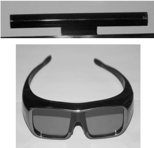
**Fig. 43.7.** Shutter glasses; infra-red transmitter mounted on a TV display
