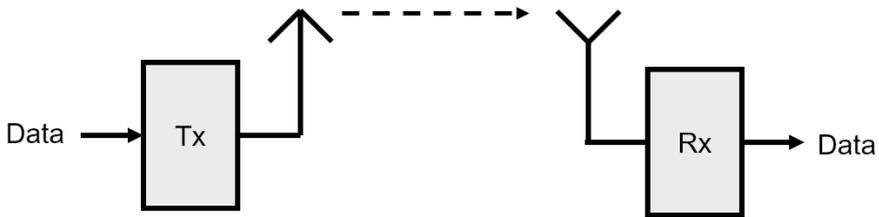
Fig. 37.35. SISO = Single Input – Single Output
