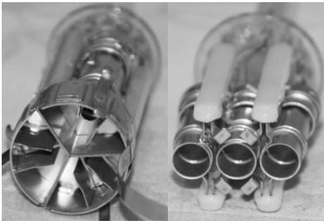
**Fig. 34.6.** Electron beam gun of a delta-type (left) and in-line-type (right) shadow mask tube
